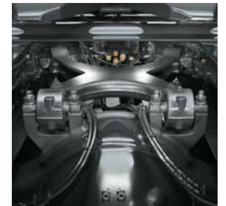
Weight-saving X control arm on the rear axle takes over the stabiliser and control arm functions.
