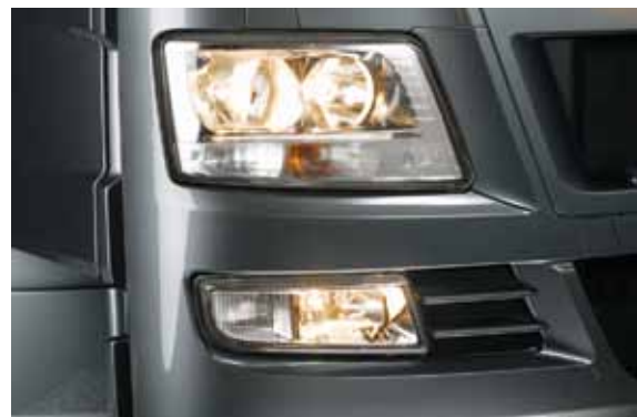
Headlights with free-form reflectors, Xenon dipped light.
